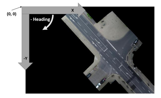
The global coordinate system used is the UTM coordinate system, as we geo-referenced our data. For easier handling of data of the same intersection in different recordings, we introduced a local UTM-like coordinate system.
