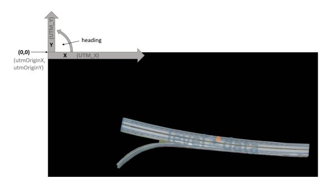
The global coordinate system used is the UTM coordinate system, as we geo-referenced our data. For easier handling of data of the same intersection in different recordings, we introduced a local UTM-like coordinate system.
